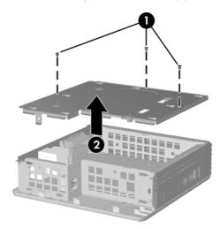
Figure 2-5 Removing the metal side cover
